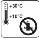
Store the battery only in a dry place at an air temperature of + 10 ° C to + 30 ° C.
