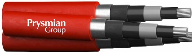
Cables with aluminium conductors for medium voltage transport and distribution of electrical energy in dry, humid or moist outdoor application, direct buried or in underground pipes or in wind applications. The cables can handle medium mechanical stresses due to their aluminum tape screen. They are designed to replace heavy and rigid cables armoured with metal in places where protection against damage is needed.
